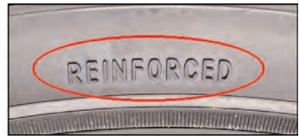
Figure 1. “Reinforced” marking on sidewall.
