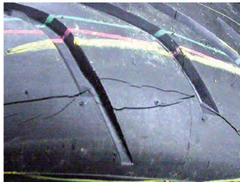
Tread cracking due to low temperatures
